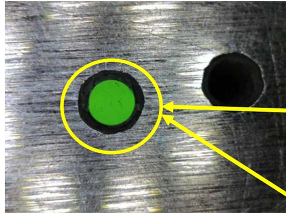
Stick the reflective tape on the end plate of module in stead of sputtering the end of fiber with mirror
