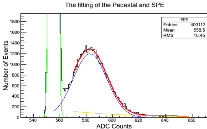
$$\text{Gain} = (\text{ADC}_{\text{signal}} - \text{ADC}_{\text{pedestal}}) \times \text{LSB} / e$$
