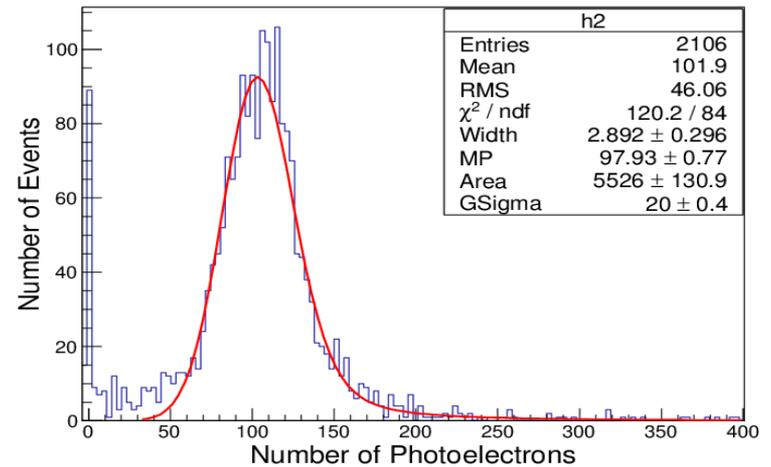
$$\text{NPE} = Q / (e \times \text{Gain})$$
