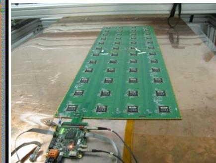
**Printed Circuit Boards (PCB)** were designed to reduce the cross-talk with 8-layer structure and buried vias.
