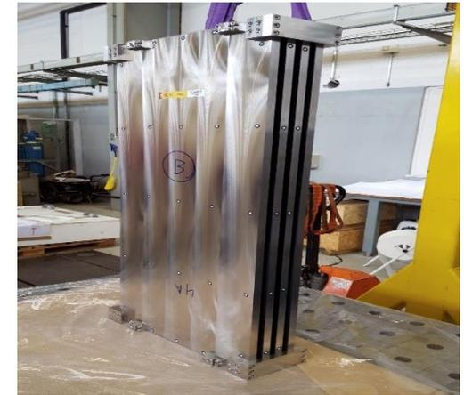
Industrial production of **flat** large absorber plates (3 m X 1 m) by **roller leveling** process
