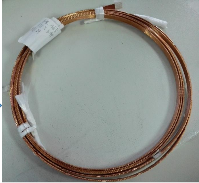
Number of strands : 18 Strand diameter : 1.2mm Materiel: Nb/Ti Complete time: 2016.2
