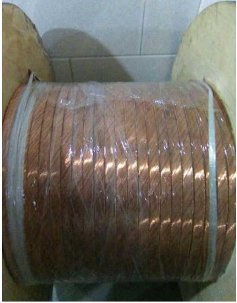
Number of strands : 32 Strand diameter : 1.2mm Materiel: Nb/Ti Tangle: 17.32 Length: » 100m RRR: » 100 Complete time: 2016.5
