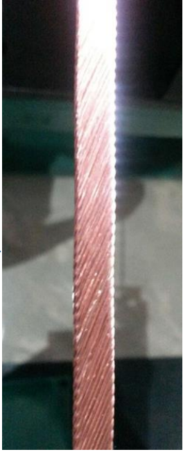
Number of strands : 17 Strand diameter : 0.727mm Materiel: Nb/Ti Complete time: 2015.7
