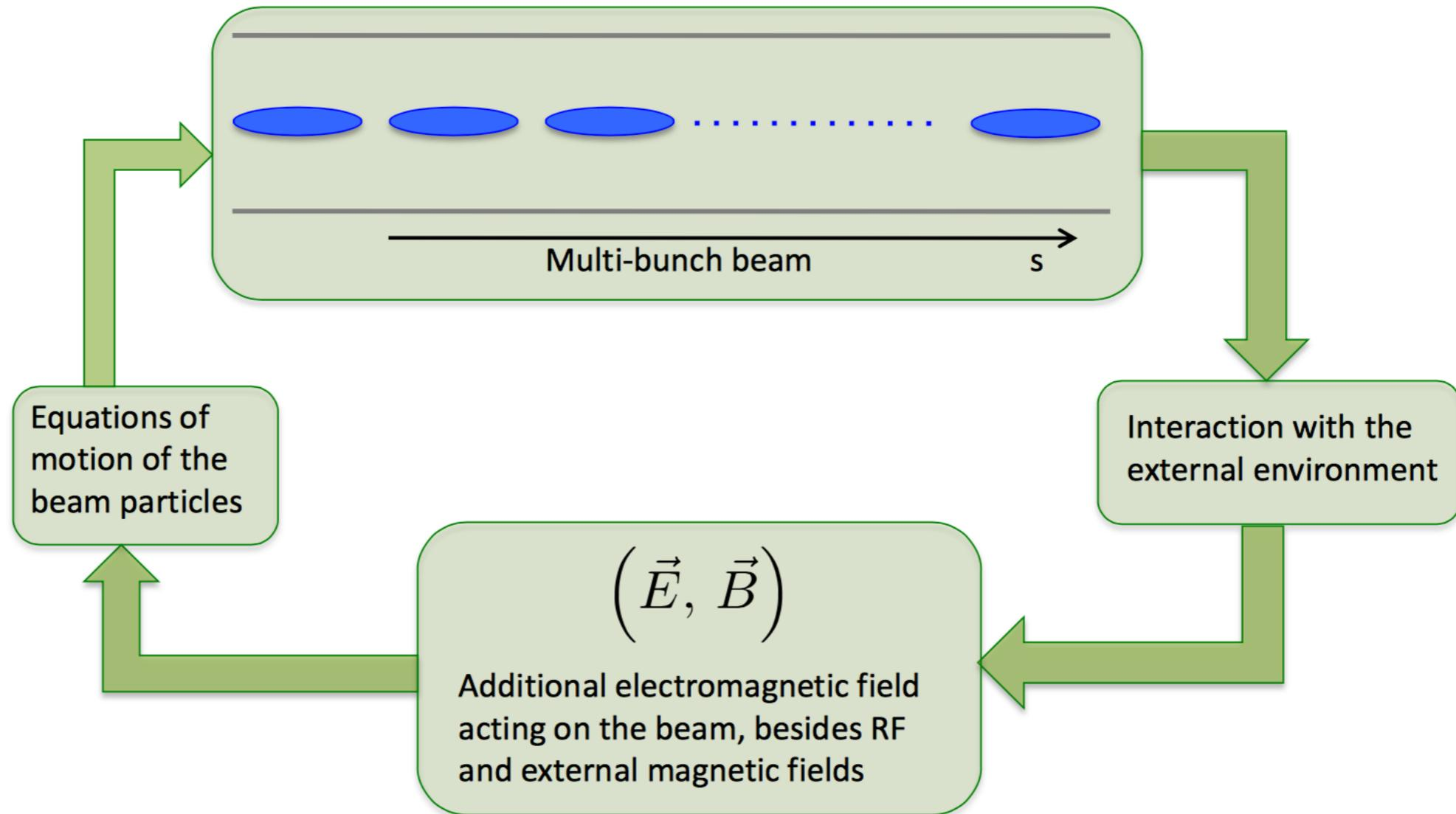
For high intensity bunches a self-consistent treatment is needed to well describe beam dynamics
