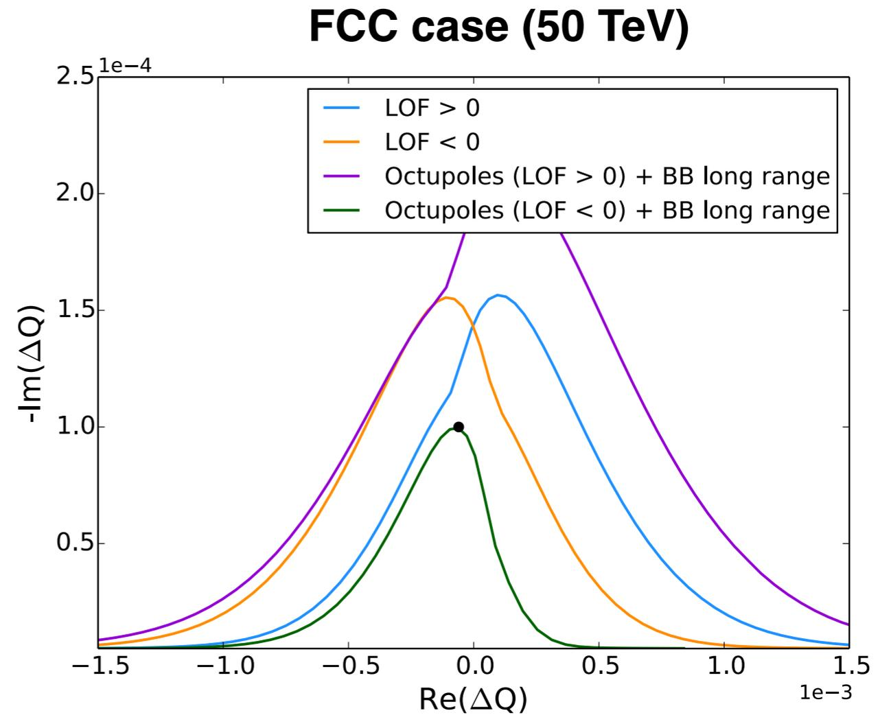
DA > 5  $\sigma$  stability diagram, Gaussian distribution is a good approximation
