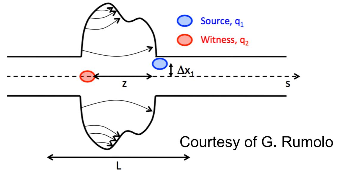
The source particle induces electromagnetic wake fields (**impedance**) that act back on the following particles modifying the electromagnetic fields provide by the lattice and RF
