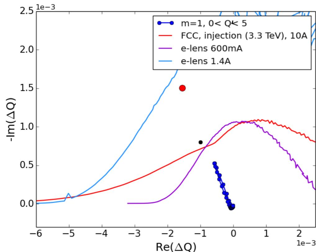
Electron lenses provide tune spread for small amplitude particles
