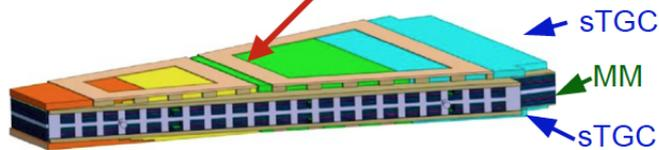
Phase-I : replace inner wheel of muon endcap with New Small Wheel – microMegas (MM) and small strip thin-gap chambers (sTGC)
