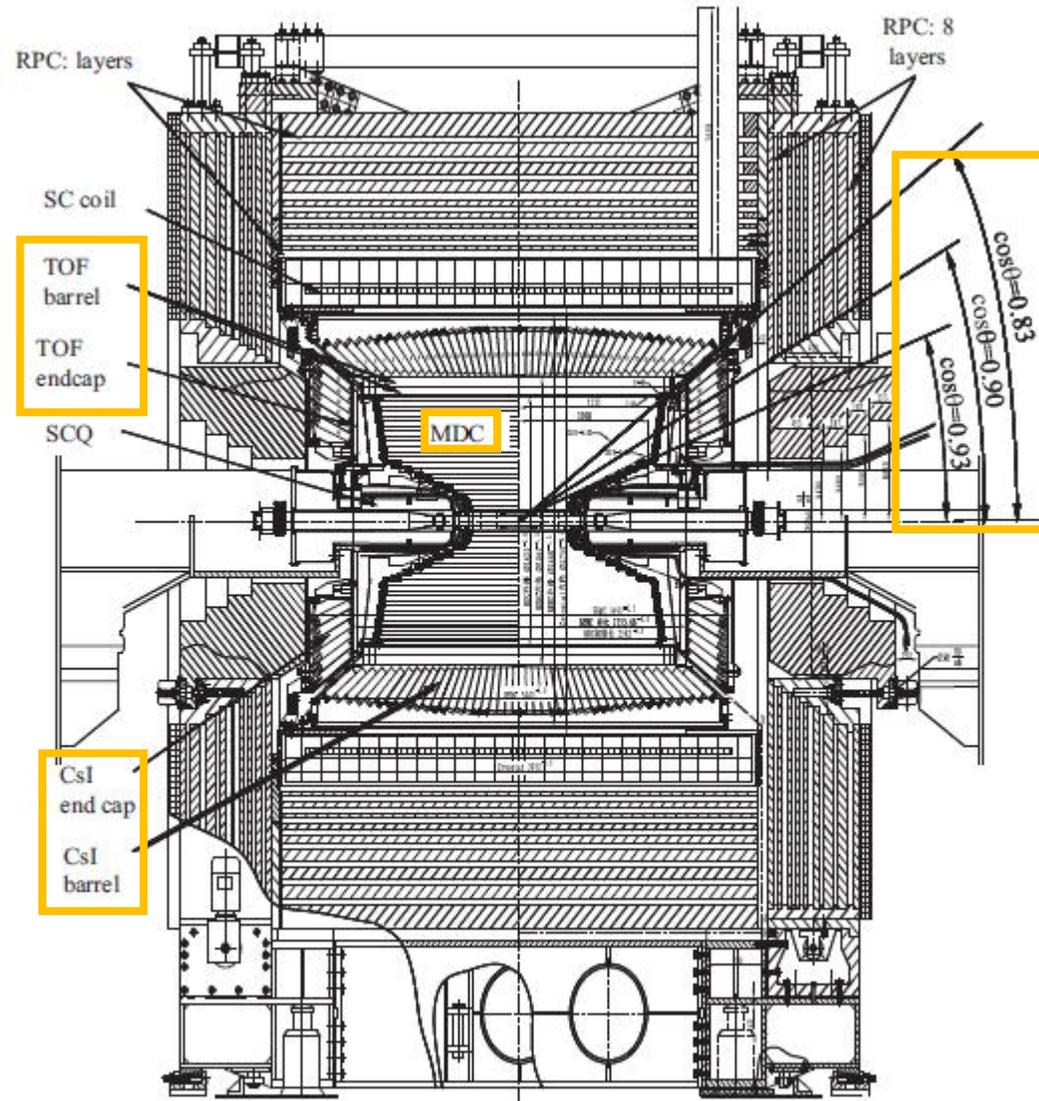
Fig. 1. Schematic drawing of the BESIII detector.
