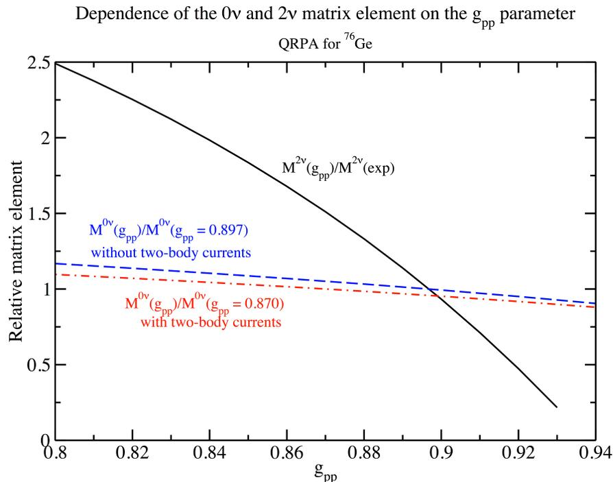
Note the steep dependence of  $M^{2\nu\beta\beta}$  on  $g_{pp}$  and the mild dependence of  $M^{0\nu\beta\beta}$ . The values  $g_{pp} = 0.897$  and  $0.870$  are the values that reproduce the experimental  $M^{2\nu\beta\beta}$  without and with 2b currents.
