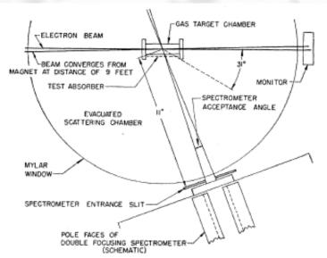
McAllister and Hofstadter 1956 188 MeV and 236 MeV electron beam from linear accelerator at Stanford
