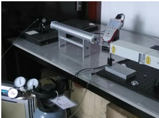
Laser performance test (laser dispersity, energy loss in argon, transmission feasibility in argon)
