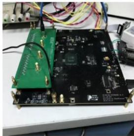
Test board: SPIROC2b chip was selected
