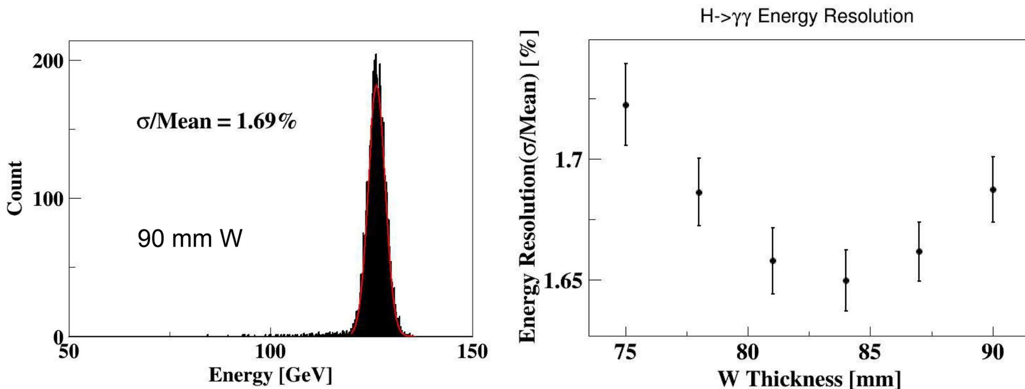
30 Layers, each layer with 0.5 mm Si + 2 mm PCB
