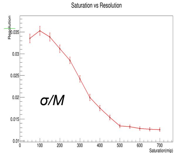
ECAL Linear Ranger: recommended to be  $>1\text{k}/1.8\text{k}$  MIP (for 10/20 mm Cell)
