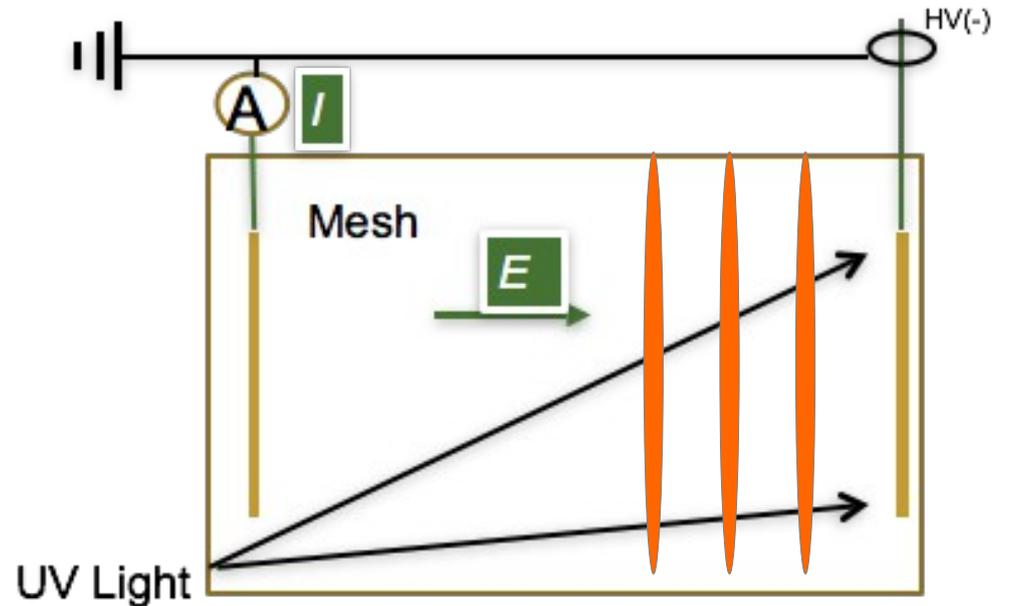
To Mimic the bunch structure & the Ion Distortion with track induced by Laser beam
