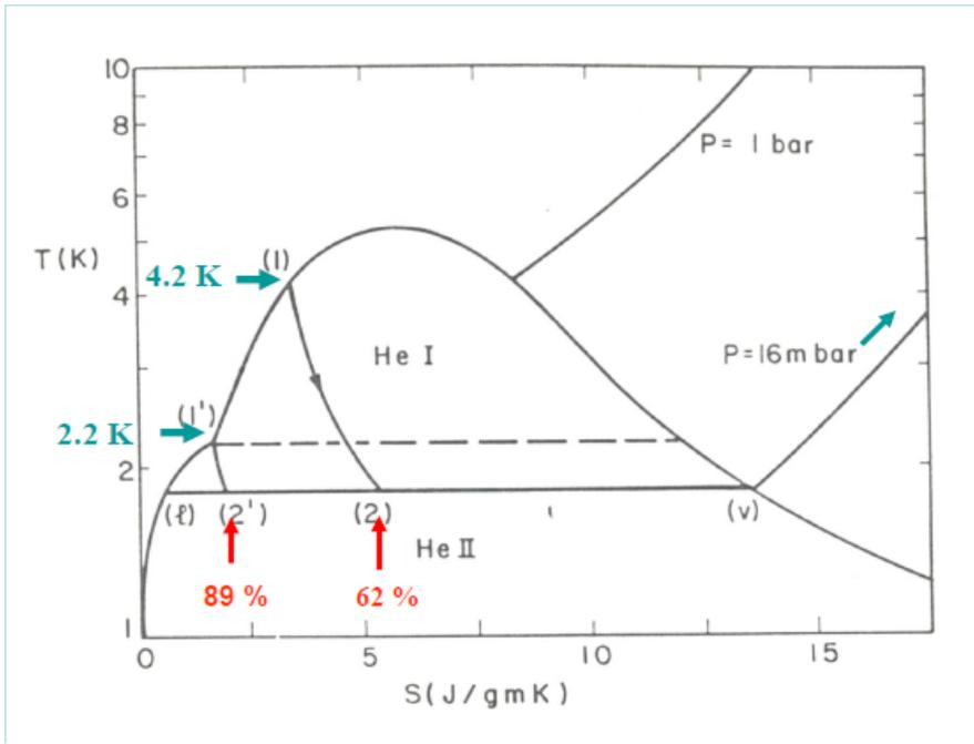
**An Efficient Heat Exchanger ( 4.2 –2K) improves the yield from 62% to 89 %**
