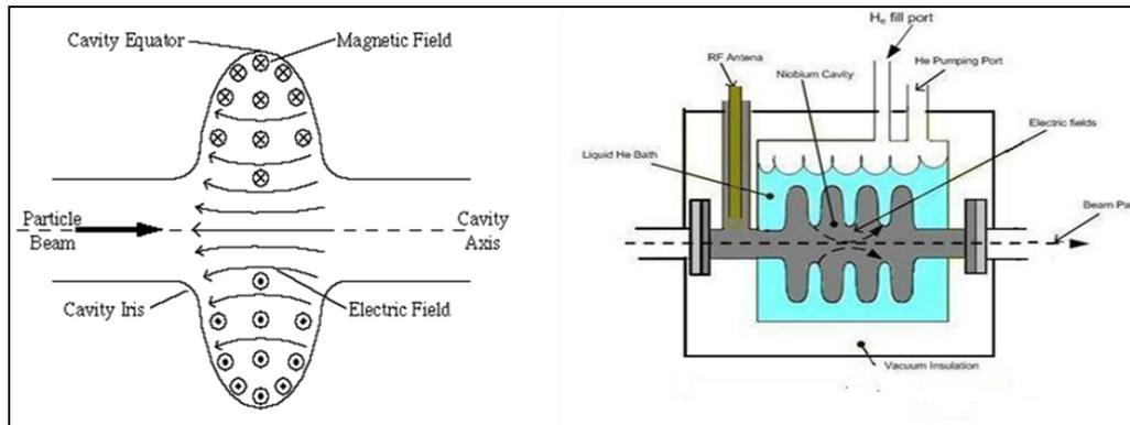
**RF POWER FEED TO THE CAVITY ( LC CIRCUIT), ELECTRIC FIELD ( MV/m) GENERATES ( Max at IRIS where Beam Passes)**
