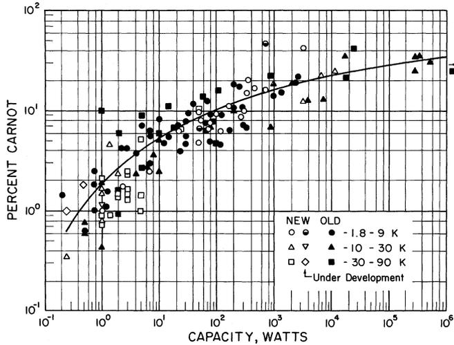
**GM Cryocooler ; 4 kW for 1W refrigeration at 4.2 K**
