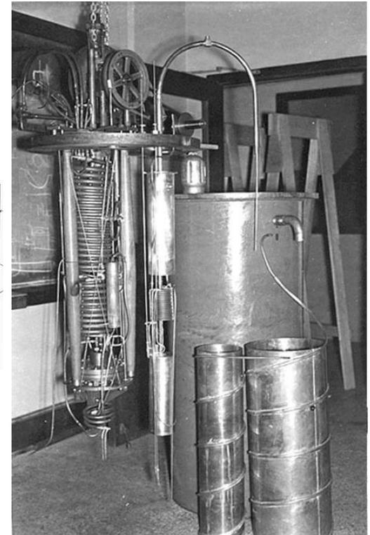
First Expender used for Helium liquefaction
