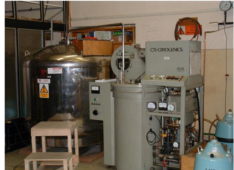
**Capacity : 10 litre/hr ( single Compressor) : Reciprocating 2 stage; 100 Nm<sup>3</sup>/hr , Reciprocating Expansion Yield = .08**
