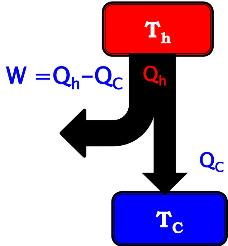
**Power ( W ) required to extract 1 W refrigeration at  $T_c$  is :  $1 / ( \text{COP} ) = \frac{W}{Q_c} = \frac{Q_h - Q_c}{Q_c} = \frac{T_h - T_c}{T_c}$**
