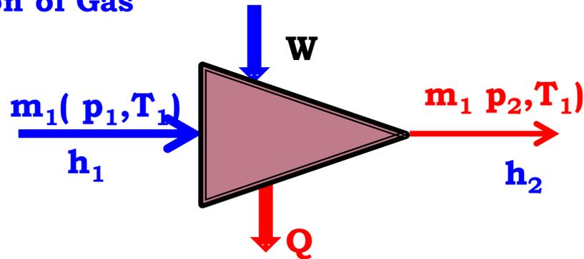
$$W = m_1 T_1 (S_2 - S_1) + m_1 (h_2 - h_1)$$
