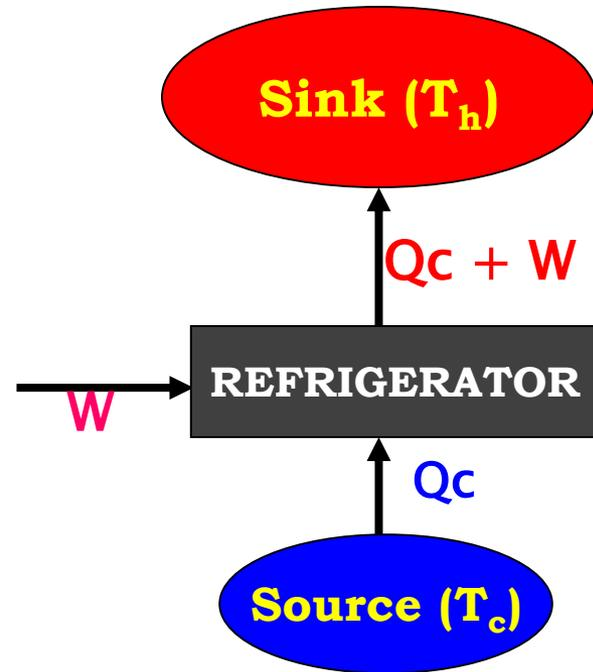
Refrigerator is analogous to Water Pump to transfer Heat ( Water ) from Lower Temp ( Lower level ) to Higher Temp ( Higher Level )
