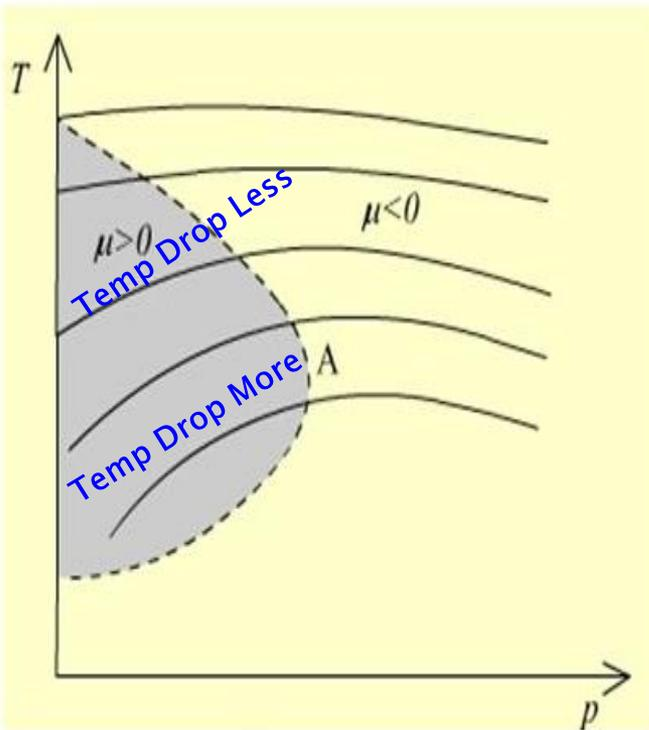
Just below their max inversion temperature drop in temperature is not significant and temperature drop increases as we lower the inlet temperature and max above their critical temperature.
