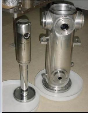
Bulk Niobium Quarter Wave RF SC Cavity ( QWR)
