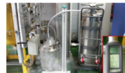
Conditioning (LN 2 absorber)
