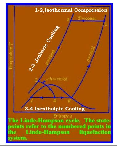
$$\frac{m_f}{M} = y = \frac{h_1 - h_2}{h_1 - h_f} \quad <<$$
