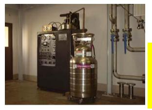
By 1946 Same Collins liquefier was commercially available in the name of ADL Collins Helium cryostat.
