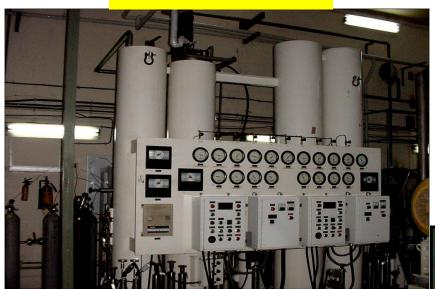
M/s CCI Helium Liquefier Capacity : 500 W or 150 L/hr Reciprocating Engine : Parallel at 60 K and 20 K Yield : 8 %, Inverse COP : 500 W/W
