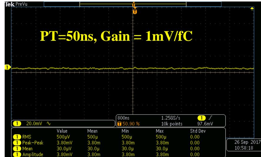
The typical intrinsic noise of sFEB is  $\sim 0.5\text{mV}$  for all gains
