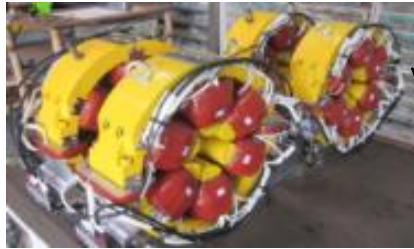
Newly installed sextupole magnets.
