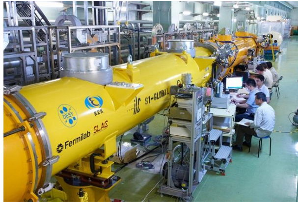
S1- Global Cryomodule Four (+4) 9-cell cavities (2010')
