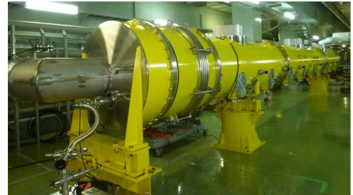
STF-2 - CM1+CM2a Cryomodule Eight + Four 9-cell cavities (2014')
