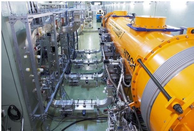
STF-1 Cryomodule Four 9-cell cavities (2008')
