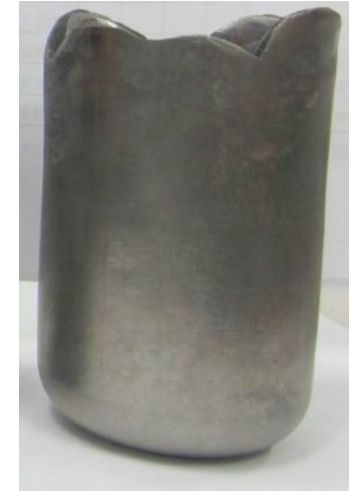
Material after deep drawing (Height > 70 mm)
