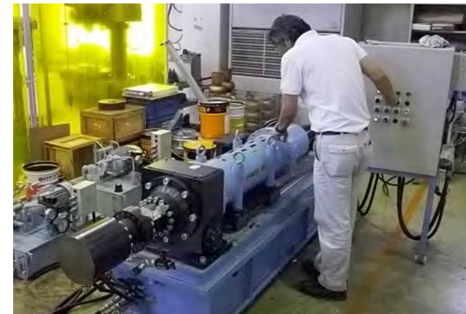
Hydroforming machine (Final hydraulic pressure: 25 MPa)
