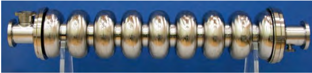
1.3 GHz TESLA-like SRF cavity for ILC (Length: 1.3 m)
