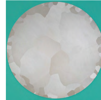
Ingot sliced Niobium (Tokyo Denkai) (Dia : 260 mm)
