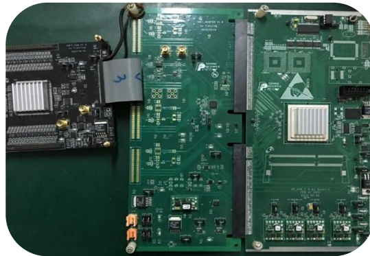
Third version of FEC ready for testing with MM
