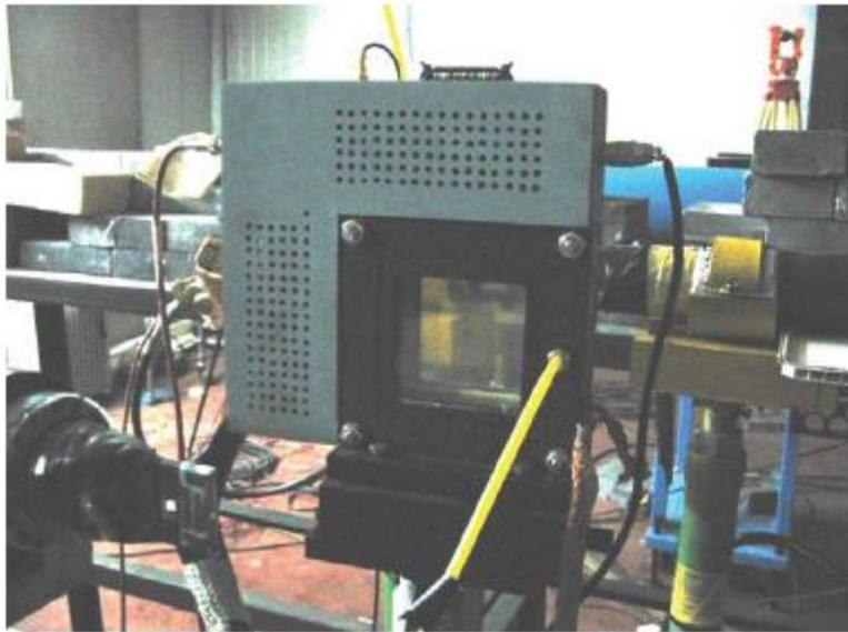
The magnetic spectrometer on E3 line which has a structure of 2Q2D, its momentum resolution is 1% and has two running modes to detect both negatively and positively charged particles. In the spectrometer the detectors contain a Cherenkov counter, TOF counters and MWPC.
