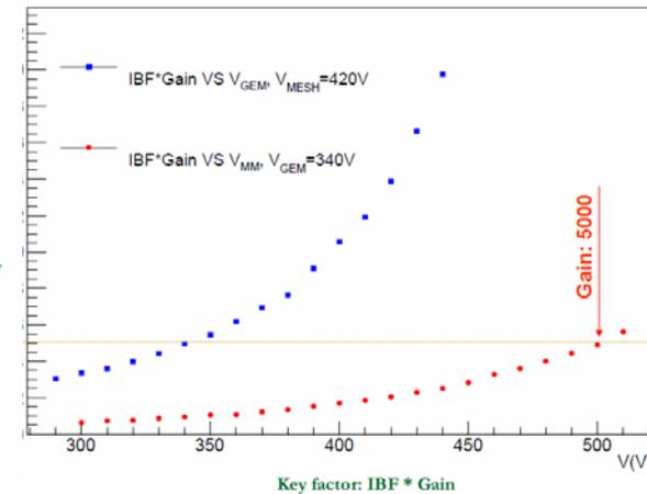
Continuous IBF prototype and IBF  $\times$  Gain
