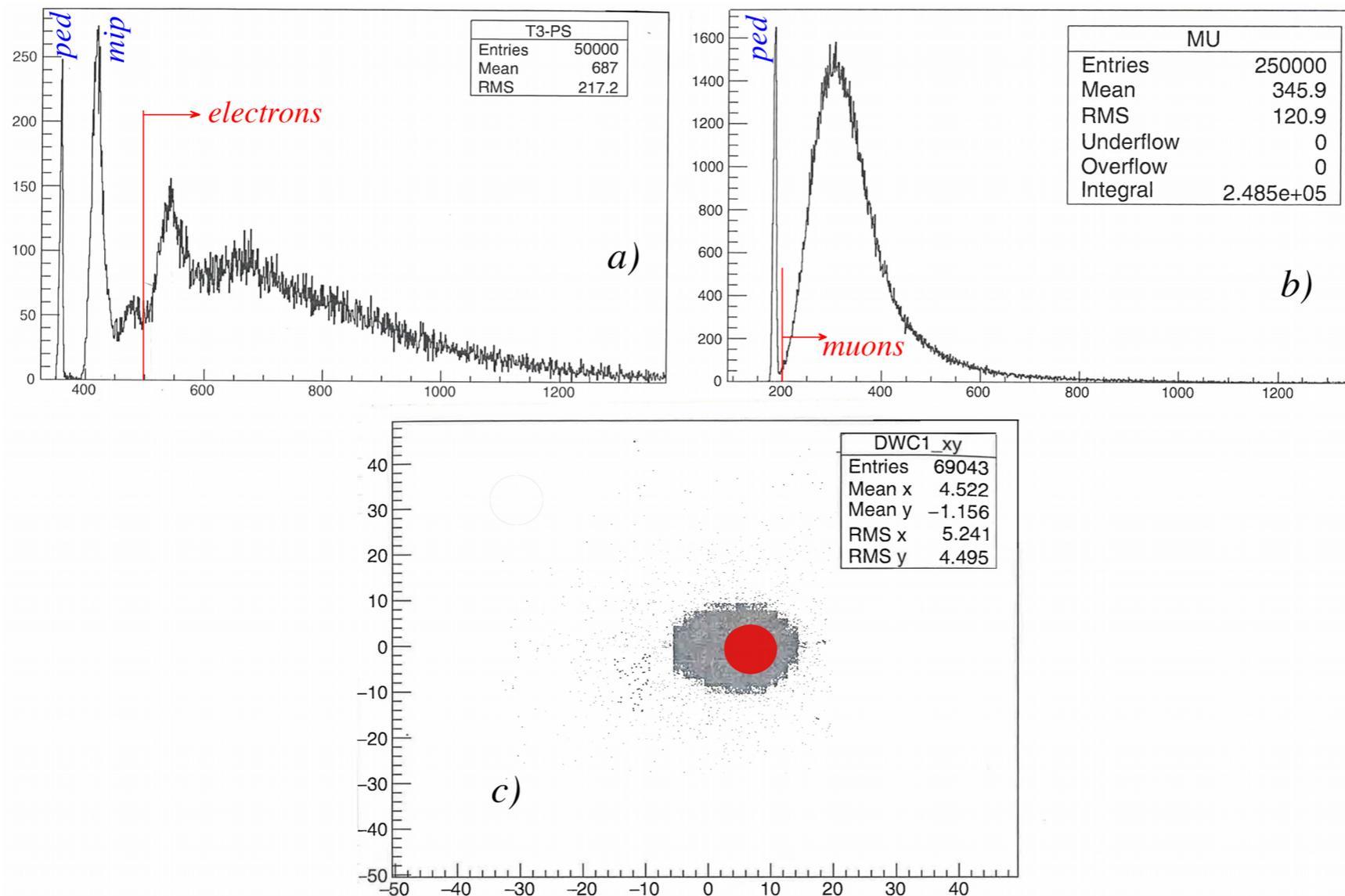
*Preshower detector and Muon counter: select electrons or muons*
