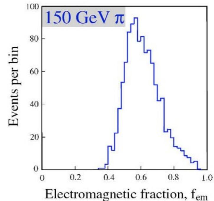
Idea: use two independent processes (scintillation and Čerenkov light emission) having very different  $e/h$  values to eliminate  $f_{em}$
