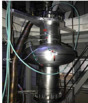
Vertical test of 650MHz 1-cell cavity
