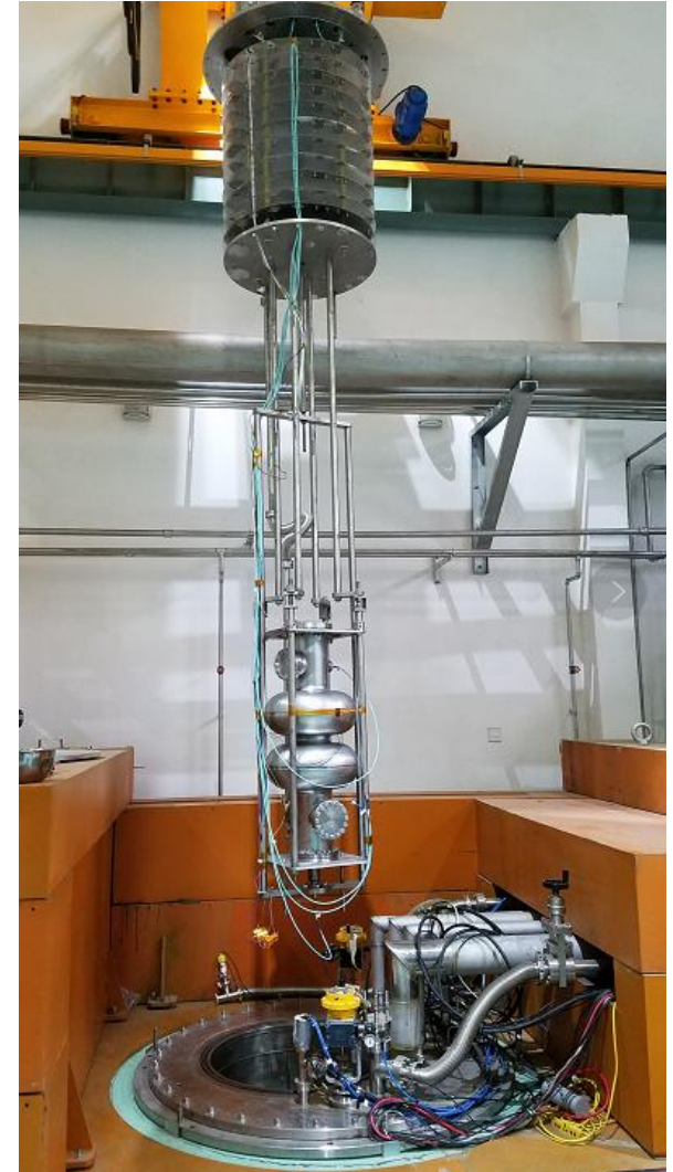
Vertical test of CEPC 650MHz 2-cell cavity
