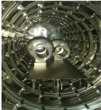
N-doping of 650MHz 1-cell cavities
