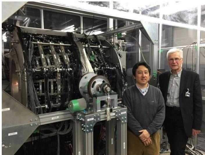
**Crystal Barrel** with CsI(Tl) :  $\sigma_{E/\bar{E}} = 2.5\% @ 1 \text{ GeV}$
