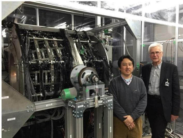
**Crystal Barrel** with CsI(Tl) :  $\sigma_{E_\gamma} = 2.5\% @ 1 \text{ GeV}$
