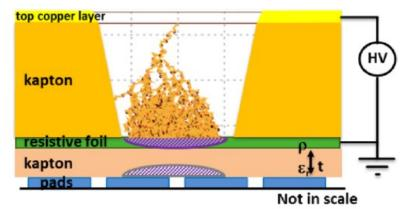
Much simpler than many other MPGDs, such as GEMs or MicroMegas Rate capability: a few tens of KHz/cm<sup>2</sup> Position resolution: ~60 µm Time resolution: 5-6 ns
