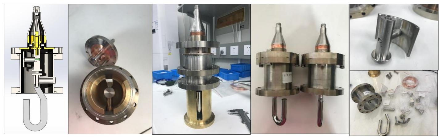
• Dismountable HOM coupler design, made of stainless steel and copper. • Different inner conductor length are used to check the transmission HOM COUPLER LOW POWER TEST
