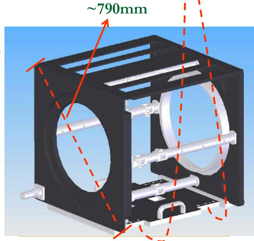
Dimension of the TPC prototype according to the PCMAG
