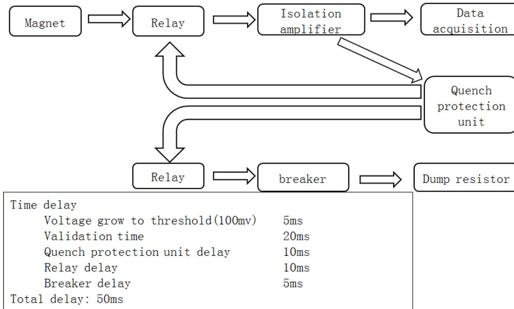
Schematic of the quench protection system
