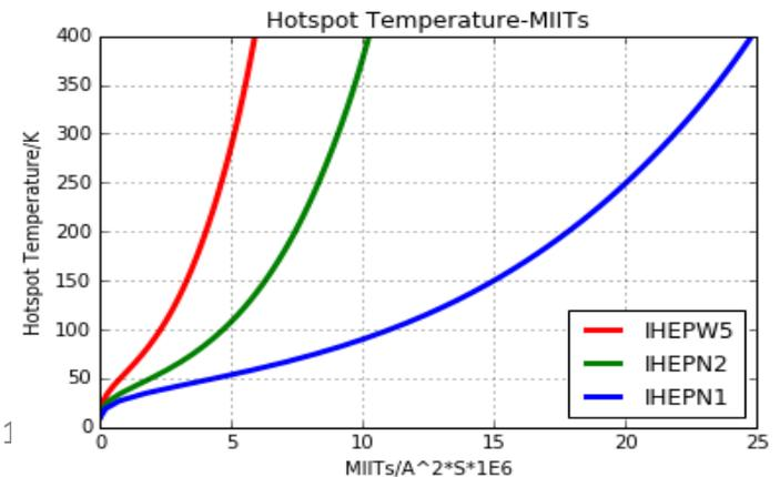
Hot spot temperature vs. MIITs for different cables
