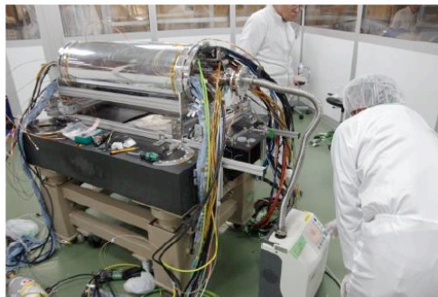
Vacuum leak check
