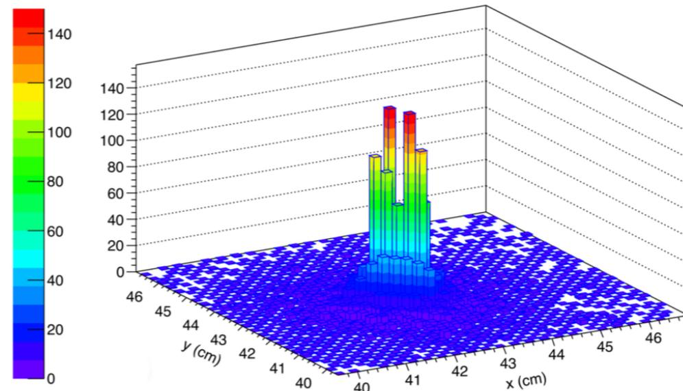
A 100 GeV  $\pi^0$  decaying 2 m before the calorimeter is identified as two electromagnetic showers.
