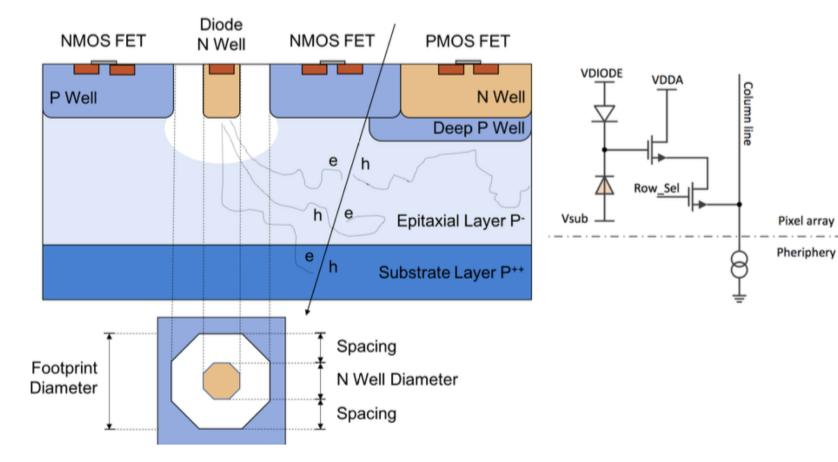
Figure 1. Cross sectional view of a CMOS pixel sensor and schematic of its in-pixel readout circuitry. Charges generated by the passing through charged particle are collected by the diode N-well mostly by diffusion.
