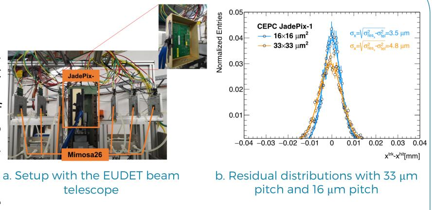
Figure 7. JadePIx-1 with the DESY test beam
