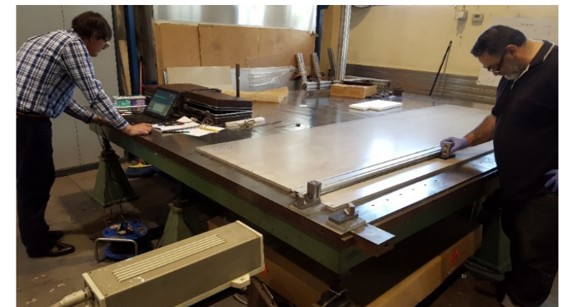
Measurement of flatness using laser interferometer
