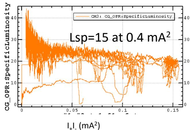
Luminosity is half at  $I_+ I_- = 0.4 \text{ mA}^2$ .
