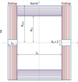
Demo of Muon Detector Geometry
