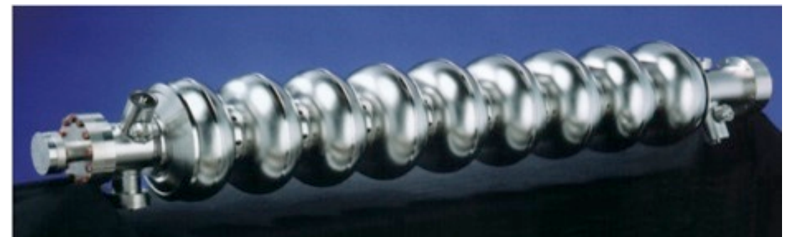
1.3GHz (L-band) SRF cavity
