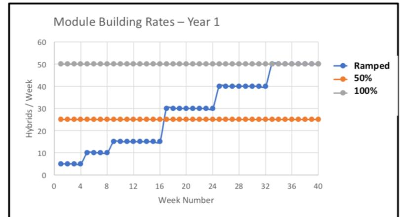
Modelling the ramping of production rates for module building
