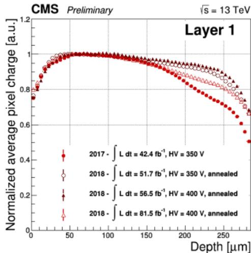
For non irradiated, fully depleted detector, the pixel charge profile (normalised average pixel charge as a function of the production depth) is expected to be flat as detector is fully efficient and all charge is collected, while for irradiated detector the losses are expected due to the trapping of carriers. The losses are larger for the charges released further from the readout plane.
