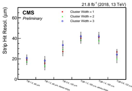
The strip hit resolution is computed by using hits in overlapping modules of the same layer ("pair method").
