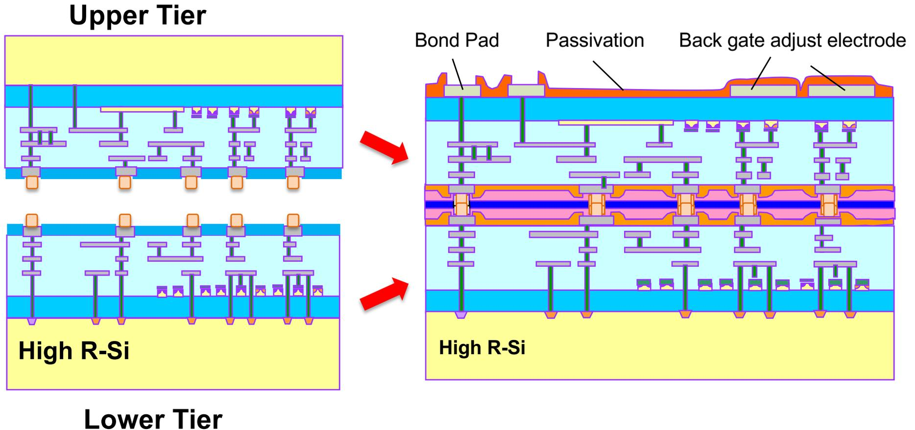
Upper and Lower Tier chips are produced in a same wafer and bonded chip to chip.
