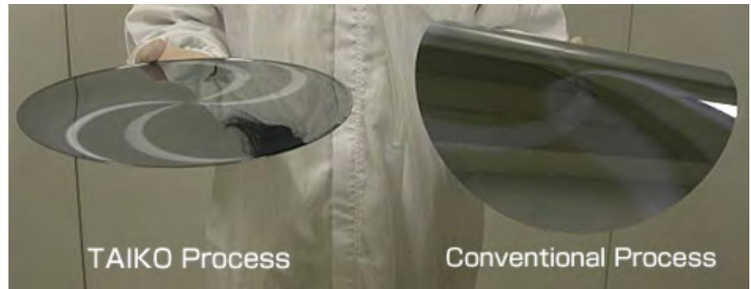
We have successfully thinned several SOI wafers to  $\sim 75 \mu\text{m}$  thick.
