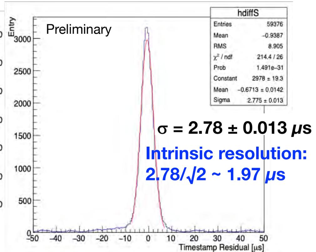
Bench test resolution is about 1  $\mu\text{sec}$ .
