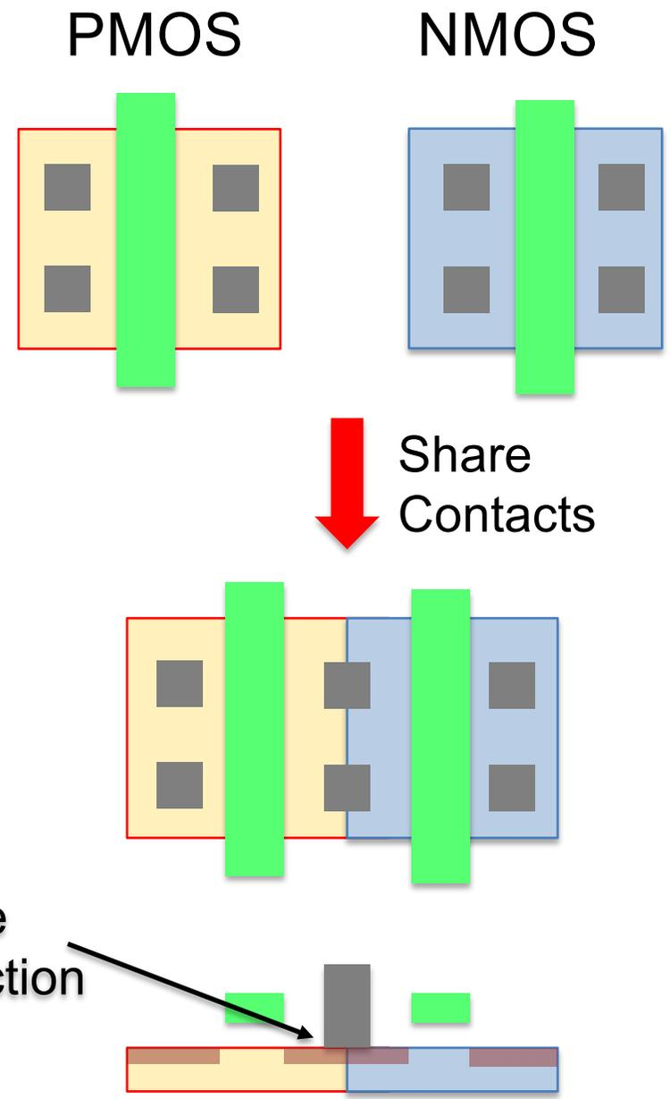
Much smaller layout is possible while keeping high analog operating voltage.
