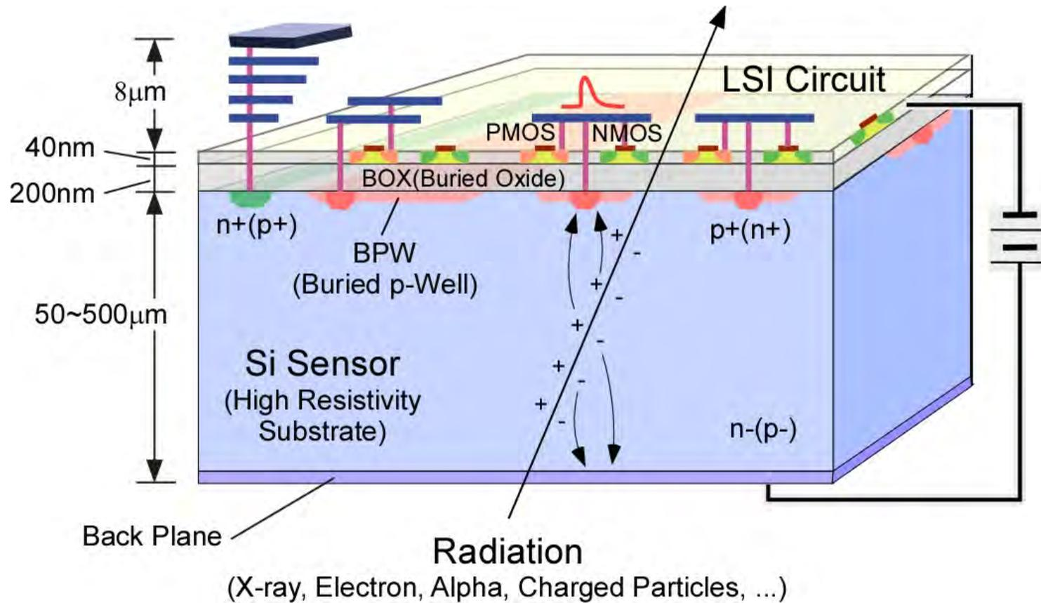
Monolithic Detector having fine resolution of silicon process and high functionality of CMOS LSI by using a SOI Pixel Technology.
