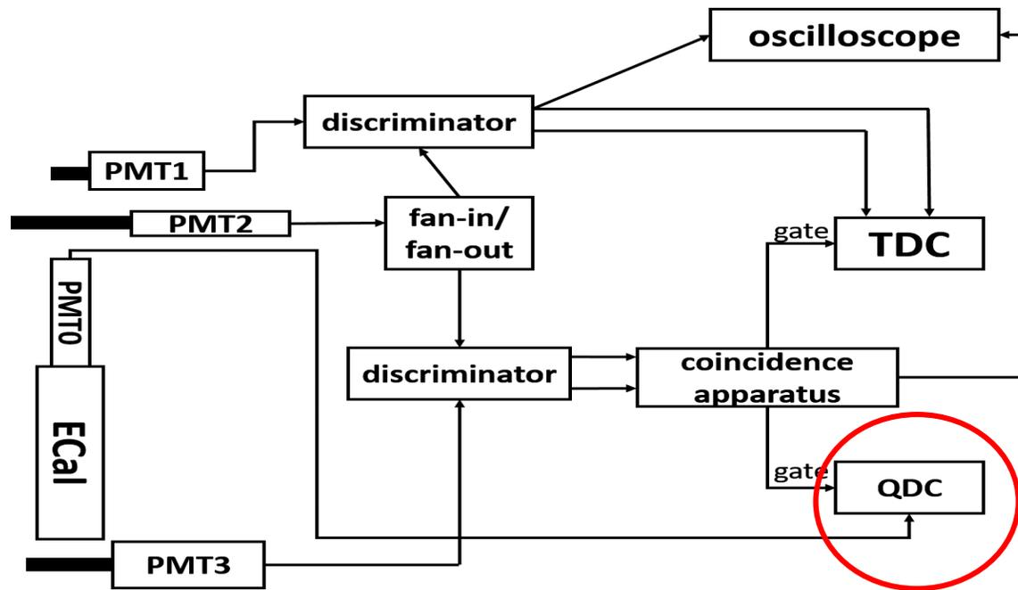
Schematic diagram of vertical cosmic ray experiment setup
