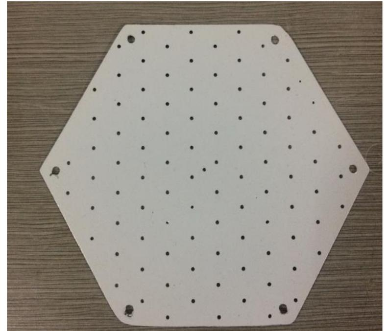
Recent test result of 5 layers shashlik test shows **half thickness** comparing with tyvek create **40% more light yield**. And this painting method will be applied to new module to check the property.
