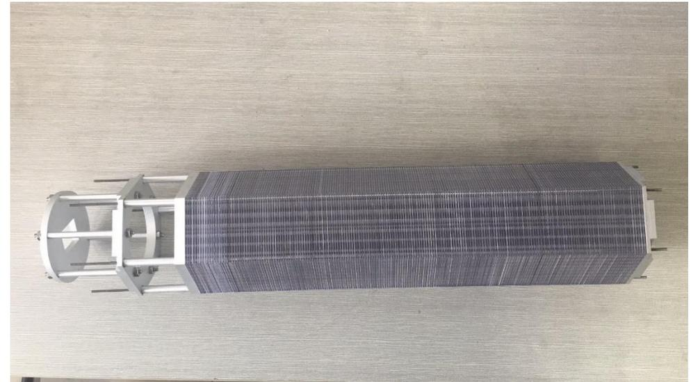
Shashlik module built as the design in support structure, which will be applied in future module.
