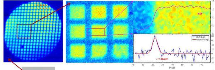
$$\sigma(\mu\text{m}) \approx 3 \text{ pixel} * \frac{90\mu\text{m}}{(1185 - 1115)\text{pixel}} = 3.9\mu\text{m}$$
