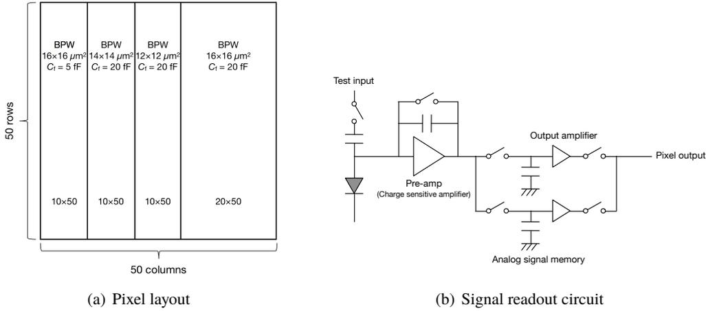
**Figure 3.** (a) Pixel array of SOFIST ver.1 with pixel size is  $20 \times 20 \mu\text{m}^2$ . Left 10 columns are for high-gain pixel, and right 40 columns are for low-gain pixel. BPW size in low-gain pixel are different for evaluating a noise. (b) Signal readout circuit in a single pixel of SOFIST ver.1. Capacitances for the analog memories are 100 fF of MIM capacitance.
