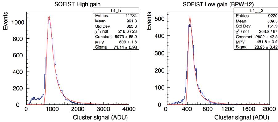
**Figure 6.** Cluster signal distributions. Left shows high-gain pixels and right shows low-gain pixels (BPW =  $12 \times 12 \mu\text{m}^2$ ). The signal readout was external 12-bit ADC.
