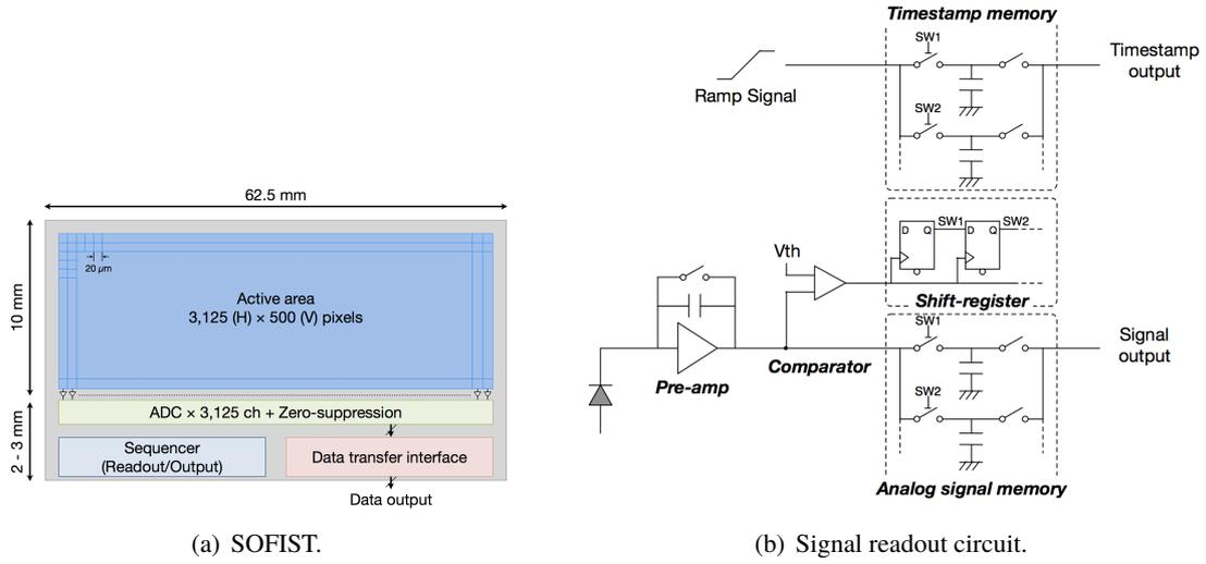
**Figure 2.** (a) SOFIST overview. Pixel size is  $20 \times 20 \mu\text{m}^2$ . Active area corresponding to  $3,125 \times 500$  pixel array is  $62.5 \times 10 \text{mm}^2$ . (b) Signal readout circuit in a single pixel. It has an amplifier, comparator, shift register, analog signal memories, and time stamp memories. A column ADC and Zero suppression logic are on the chip.
