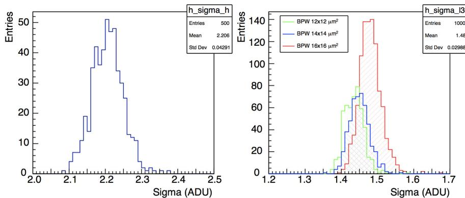
Figure 5. Pixel noise distribution. Left shows high-gain pixels and right shows low-gain pixels. The signal readout was done with an external 12-bit ADC.
