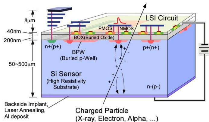
**Figure 1.** Cross section of the SOI monolithic pixel detector. The signal readout circuit is processed on the SOI layer. The buried oxide layer (BOX) isolates the readout circuit from the silicon sensor. The buried  $p$ -well (BPW) is created under the BOX to suppress the back-gate effect. The BPW is also utilized as a sense node to collect charges in the sensor. Thickness of the silicon sensor can be reduced from  $500\ \mu\text{m}$  to  $50\ \mu\text{m}$  according to application.
