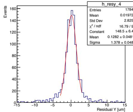
**Figure 7.** Residual distribution in  $y$ -direction to the track reconstructed by four layers of FPIX2.
