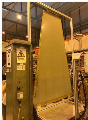
Figure 8.3: Top) Picture of the CMS GE1/1- \mu RWell prototype. Bottom) Picture of the CMS GE2/1 sector with two M4 \mu RWell prototypes.
