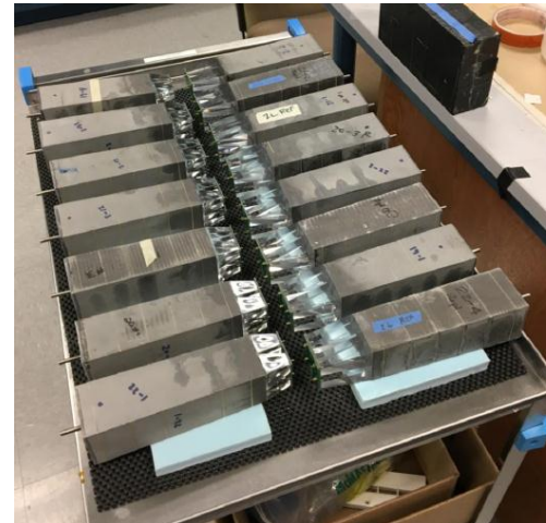
2D projective blocks for the large \eta prototypes
