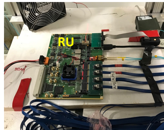
4 sensors Connected to one RU
