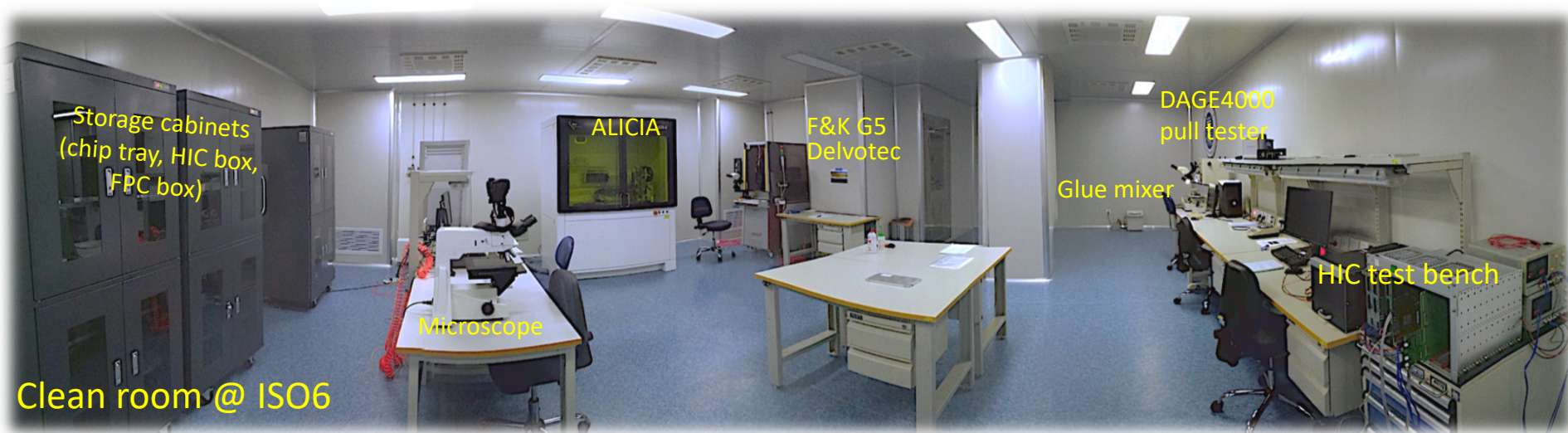
ALICE/ITS Chip Design/Testing (CCNU) : Chaosong, Ping, Mangmang, Shuguang
