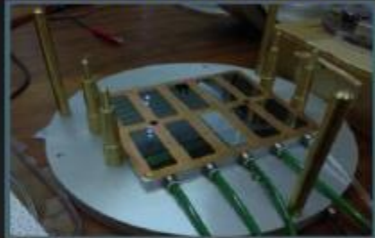
VELO sensor tiles testing device
