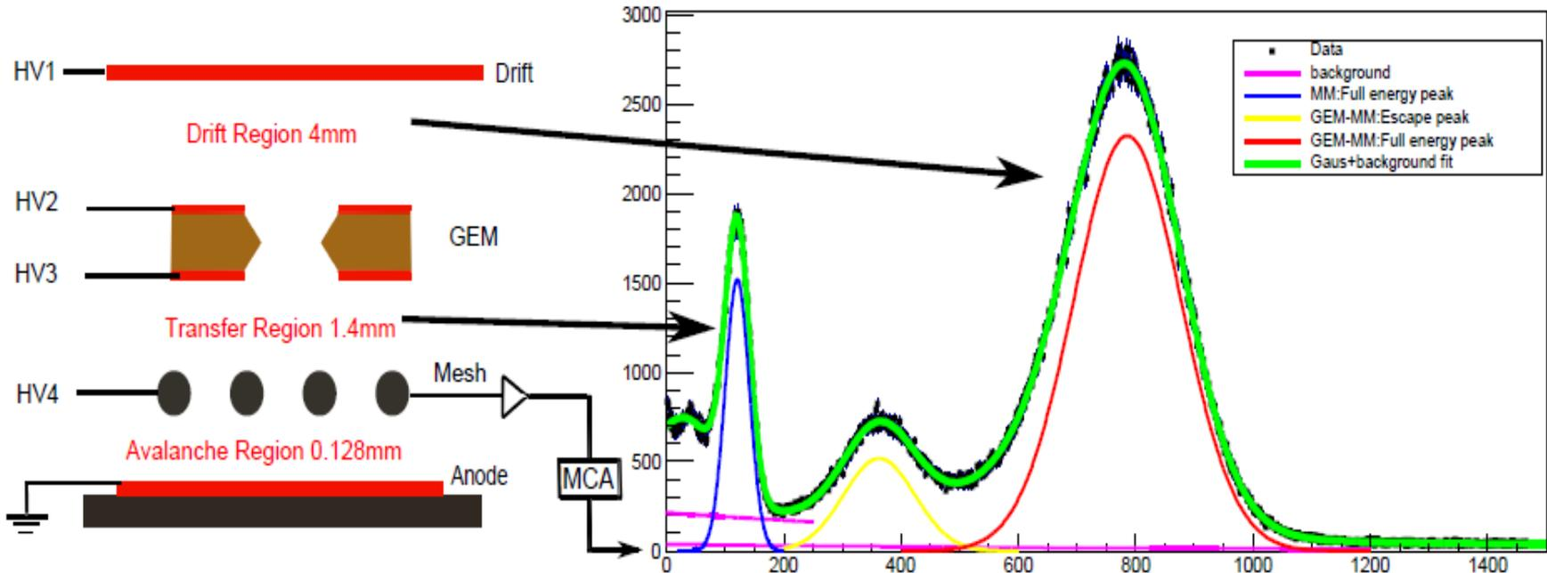
**GEM-MM configuration(left) and pulse height spectrum on 5.9 keV for a GEM-MM showing each peak and the corresponding location of primary ionization(right)**
