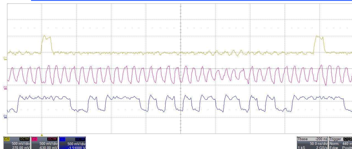
SLVS SPI-interface @ 160Mbps, 实测验证√
