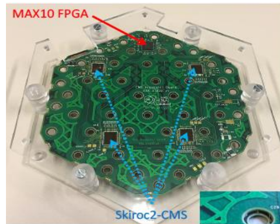
SKIROC 2 ASIC developed by OMEGA group designed for ILC. Not the final front-end chip for CMS.
