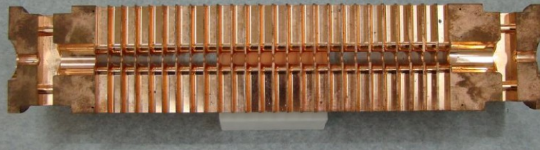
accelerating structure high gradient makes machine cheap
